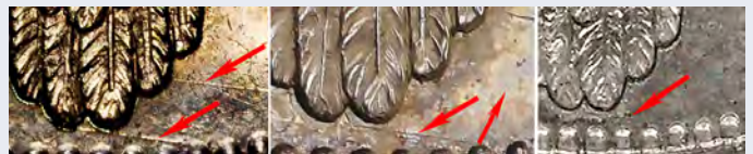
Figure 7. Fading die lines around eagle’s tail feathers.
