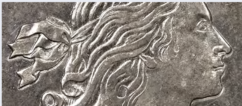
Figure 5. Greatly reduced portrait rust on Linderman Class III. Note that the outlines around face and ribbons are a result of double-striking.
